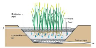
Figure 22. Schematic cross-section of a VFB (source: Morel and Diener, 2006)<sup>18</sup>. The middle layer of coarse sand typically has a height of 50 cm, the top gravel layer a height of 10 cm.
