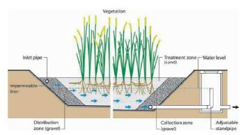
Figure 18. Schematic cross-section of a HFB (source: Morel and Diener, 2006).
