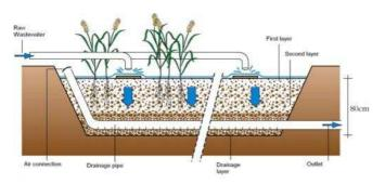
Figure 25. Pre-treatment of raw wastewater in the first stage (a VFB) of the French System (source: Molle et al., 2005). Wastewater flows out of the *end* of the distribution pipes (*without* small holes along the pipe length).
