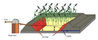
Figure 19. Schematic cross-section of a HFB showing pre-treatment with a septic tank on the left (source: Fehr, 2003).
