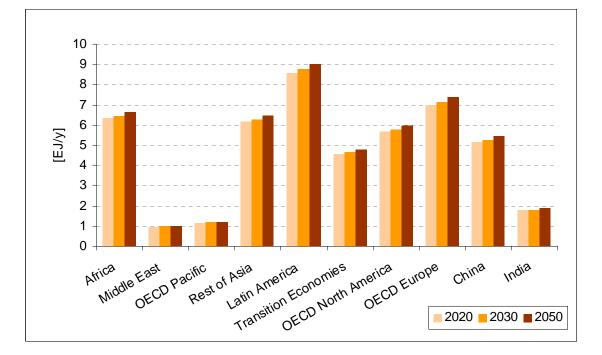
Figure 4 provides the technical potential for hydropower at a regional level. High potentials can be found in Asia and Latin America. The global technical potential amounts to 50 EJ/y.
