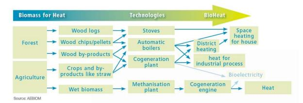
Figure 3-3: Biomass chains for biomass heat production (EREC 2007)
