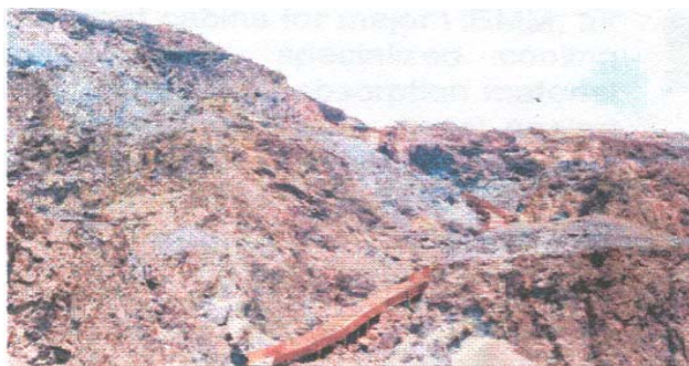
Discharge of mine water through steel launders
