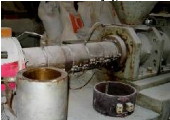
Heaters of extruder machine without heat insulation
