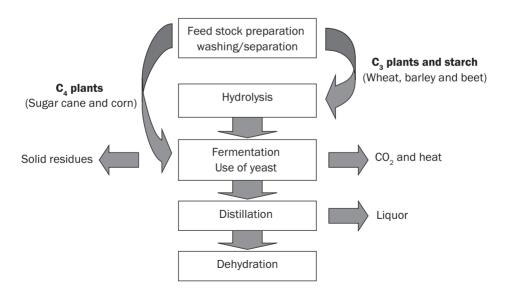
Figure 1. Production process of ethanol (Barriga, 2003).
