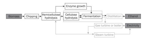
Figure 4. Generic process scheme for the production of ethanol from lignocellulosic biomass.
