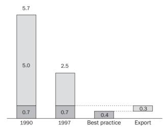
Figure 8. Evolution of water consumption in industrial ethanol production from sugarcane (m³/ton of sugarcane). Source: Dedini (2008).
