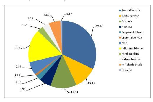
\* MEK: Methyl Ethyl Ketone Figure 4.30 Carbonyl emissions from BS III Diesel +B10 fueled in HCV (mg/kW.hr)
