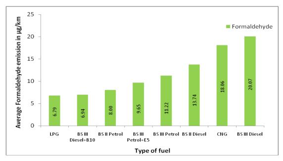
Figure 4.39 Comparison of formaldehyde emission from various fuels in three wheeler
