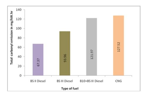
Figure 4.32 Comparison of total carbonyl compound emissions using various fuels in HCV
