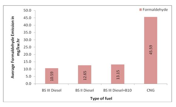
Figure 4.41 Comparison of formaldehyde emission from various fuels in LCVs
