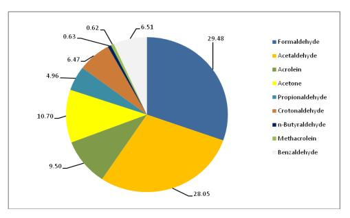
Figure 4.29 Carbonyl emissions from BS III Diesel fueled in HCV (mg/kW.hr)
