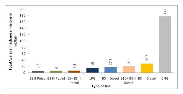
Figure 4.35 Comparison of Average methane emissions using various fuels in four wheeler category
