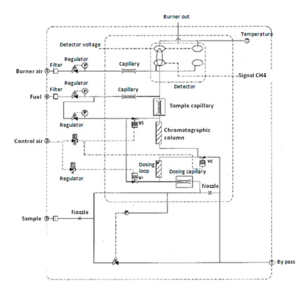
Figure 3.2 Flow diagram of FID 4000 LCG measurement system
