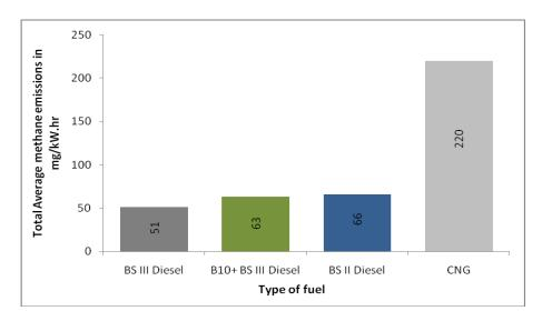
Figure 4.37 Comparison of methane emissions using various fuels in HCVs
