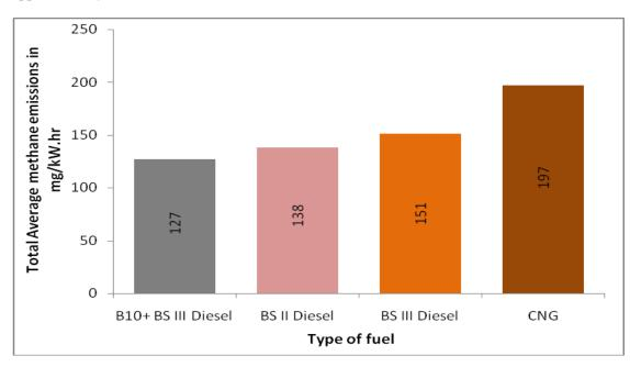
Figure 4.36 Comparison of Average methane emissions using various fuels in LCVs
