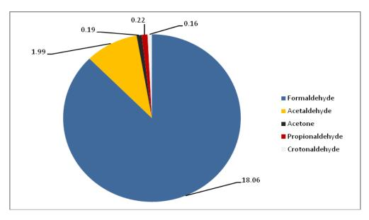
Figure 4.7 Carbonyl emissions from CNG fueled three wheeler (µg/km)
