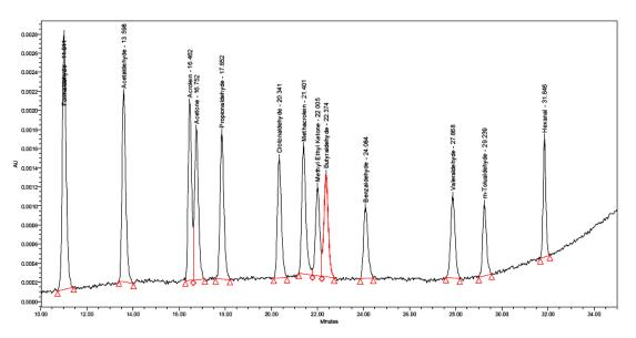
Elution of profile of the target carbonyl-hydrazone from the supelcosil HPLC Column
