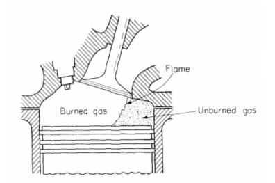
Figure 2.1 In-cylinder burned gas and unburned gas formation
