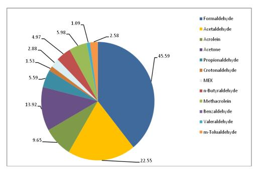
\* MEK: Methyl Ethyl Ketone Figure 4.26 Carbonyl emissions from CNG fueled LCV (mg/kW.hr)
