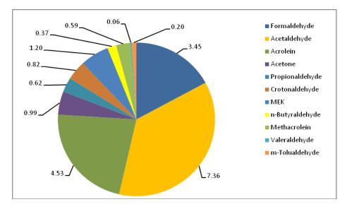
\* MEK: Methyl Ethyl Ketone Figure 4.18 Carbonyl emissions from LPG fueled in four wheeler passenger cars (µg/km)
