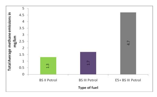
Figure 4.33 Comparison of methane emissions using various fuels in two wheeler category
