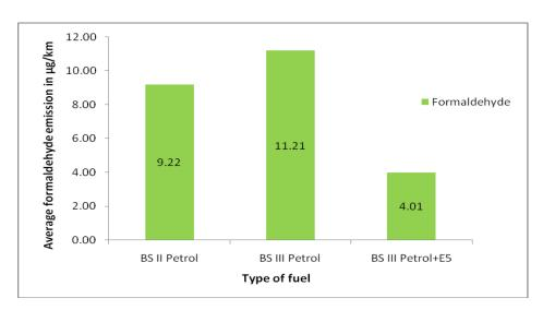
Figure 4.38 Comparison of formaldehyde emission from various fuels in two wheeler.
