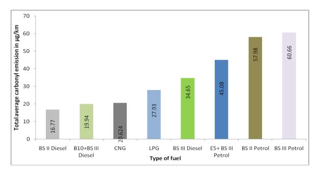
Figure 4.13 Comparison of Average total carbonyl compound emissions using various fuels in three wheeler category
