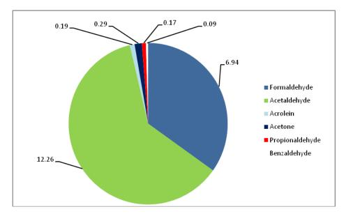
Figure 4.8 Carbonyl emissions from BS III Diesel+B10 fueled three wheeler (µg/km)
