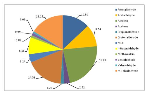
\* MEK: Methyl Ethyl Ketone Figure 4.24 Carbonyl emissions from BS III Diesel fueled LCV (mg/kW.hr)
