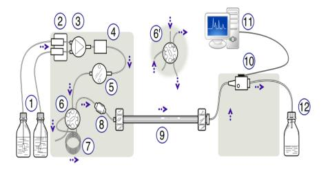
Figure 3.3 Schematic representation of an HPLC unit
