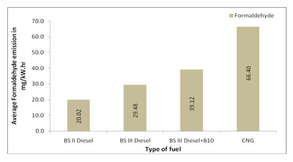
Figure 4.42 Comparison of formaldehyde emission from various fuels in HCVs
