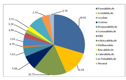
Figure 4.28 Carbonyl emissions from BS II Diesel fueled in HCV (mg/kW.hr)
