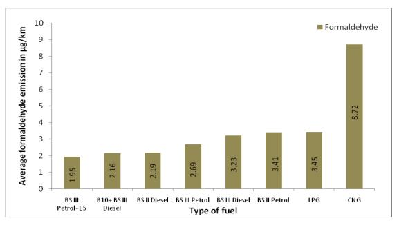
Figure 4.40 Comparison of formaldehyde emission from various fuels in four wheeler
