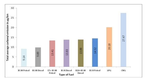
Figure 4.22 Comparison of Average total carbonyl compound emissions using various fuels in four wheeler passenger car category
