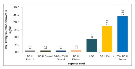
Figure 4.34 Comparison of Average methane emissions using various fuels in three wheeler category
