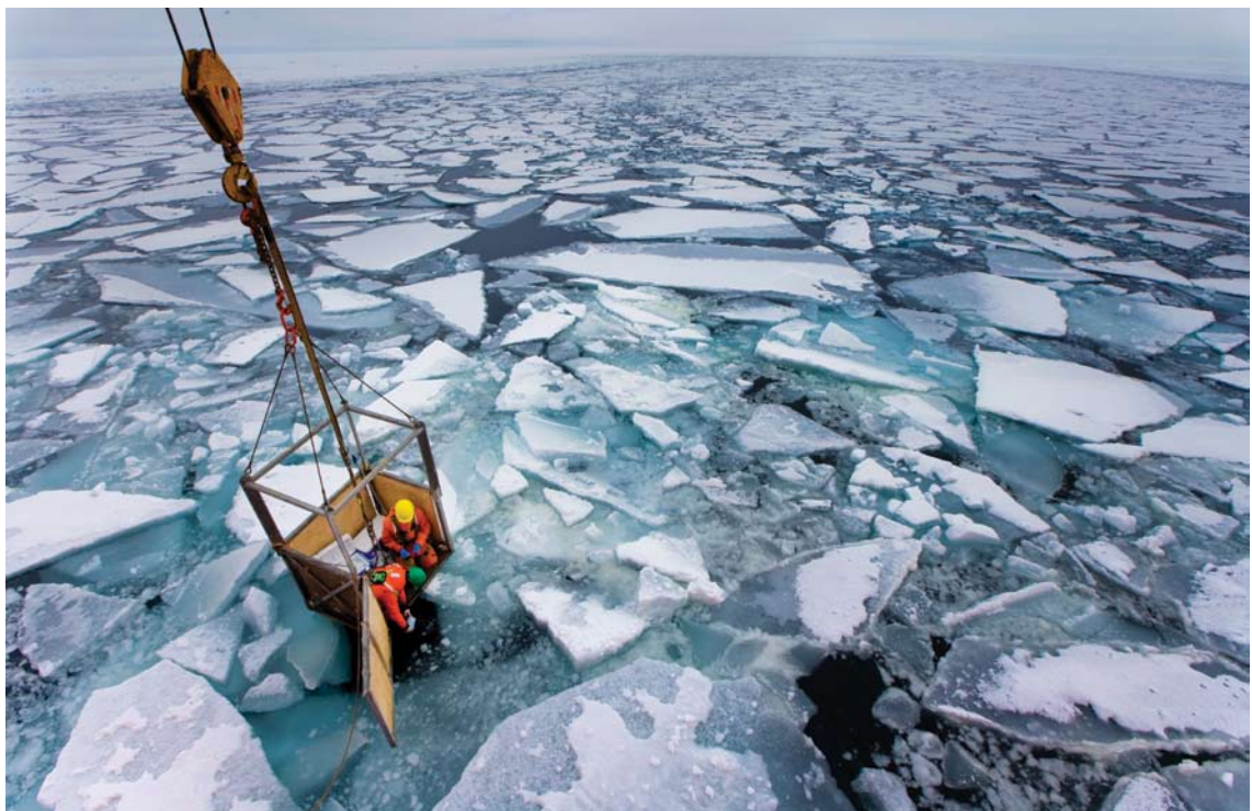
Collecting samples of young ice and seawater from a crane cage of the Canadian research icebreaker Amundsen to investigate the behaviour and transport of mercury in the Arctic Ocean
