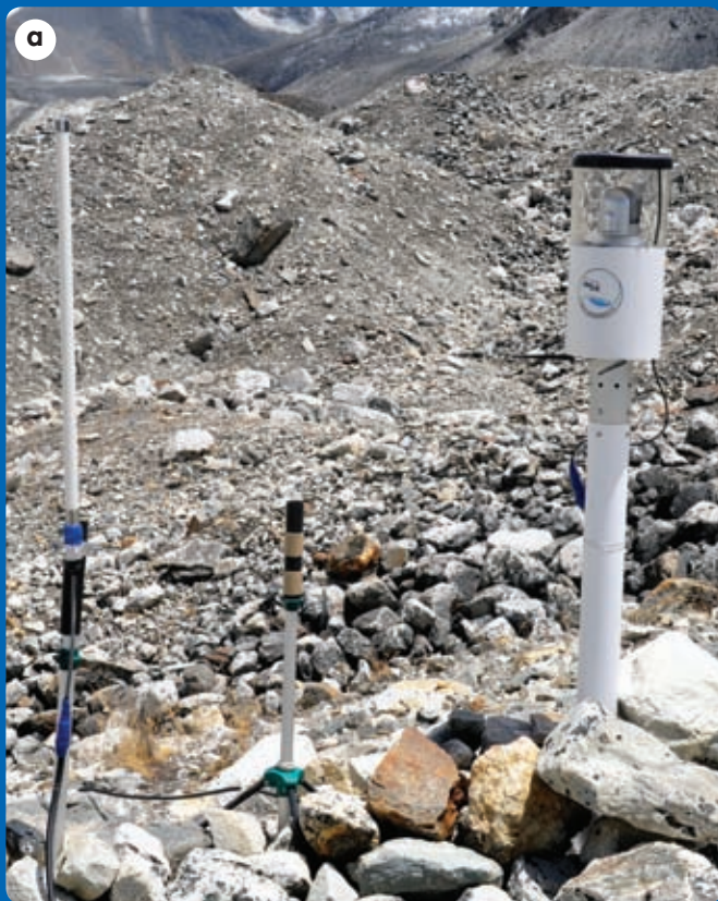
Figure 6: Monitoring of Imja glacial lake: a) field server the lake (2009); b) solar panel for field server (2009); c) part of image from field server at lake (26 June 2009); d) part of image from field server at Namche Bazar (1 Jan 2010)
