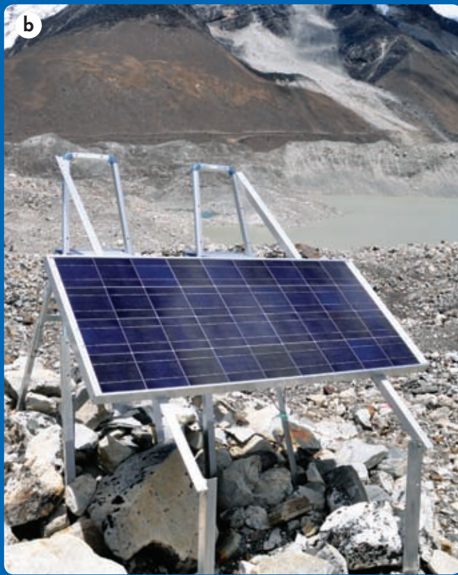
Figure 6: Monitoring of Imja glacial lake: a) field server the lake (2009); b) solar panel for field server (2009); c) part of image from field server at lake (26 June 2009); d) part of image from field server at Namche Bazar (1 Jan 2010)
